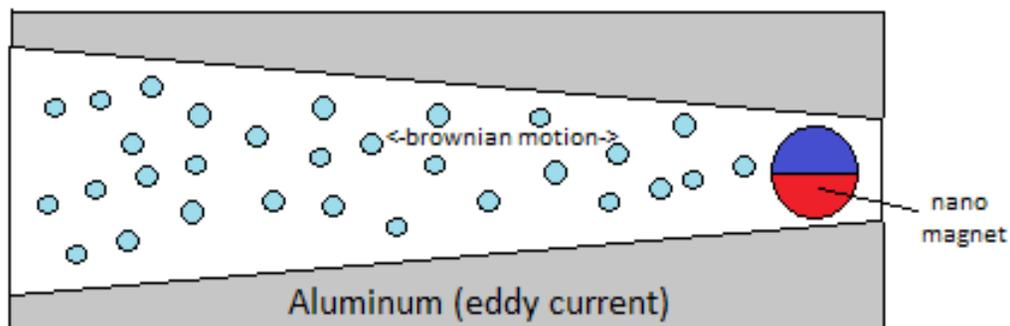
A nano magnet vibrates due to brownian motion in a fluid such as water. If this nano magnet is placed into a device with aluminum in it, the nano magnet will interact with the aluminum and cause eddy currents. In this device shown above the aluminum is shaped in a sideways V. The narrower gap causes more eddy current braking or dampening to occur.
